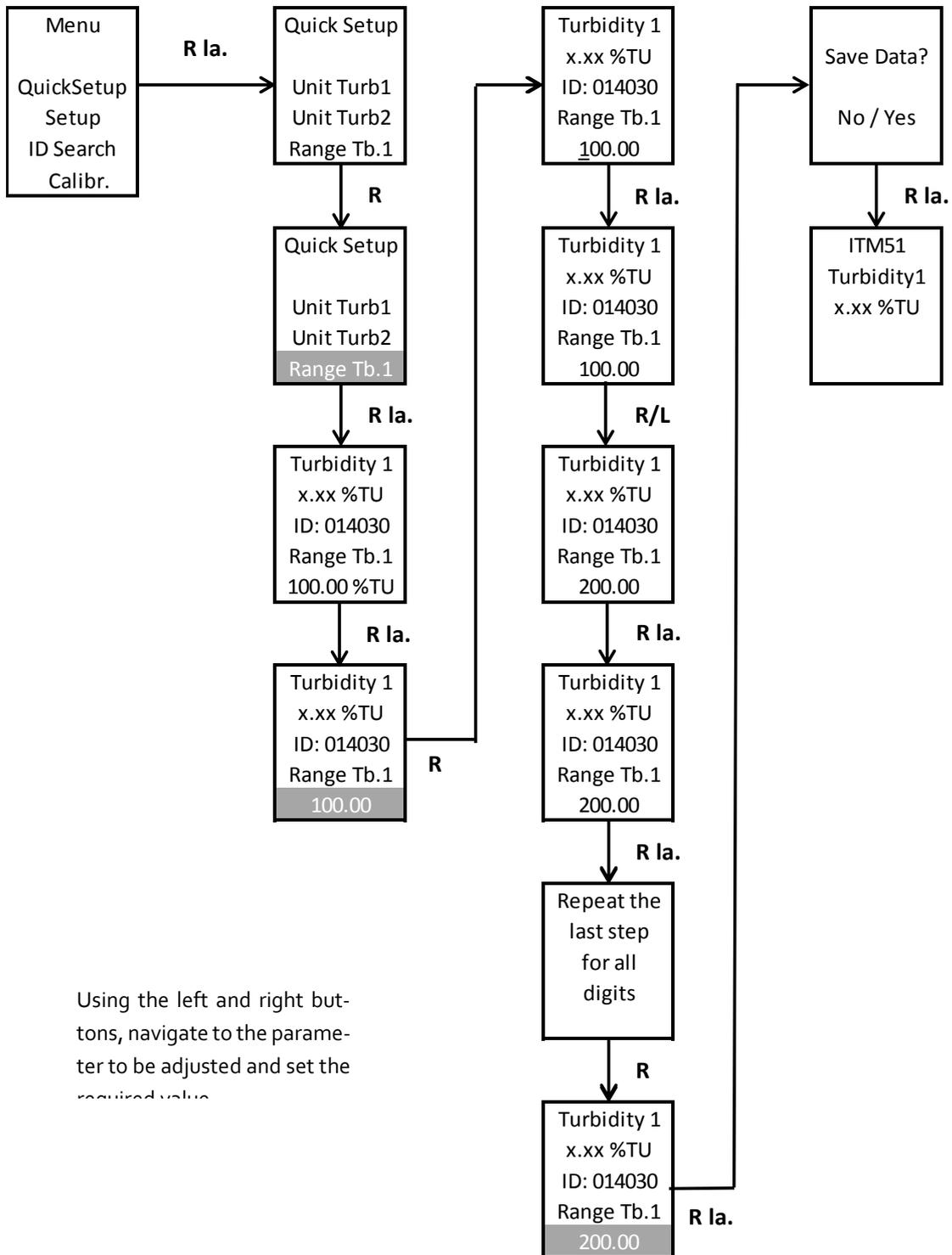
Alternative to entering the measurement range as described above, the measurement range can also be adjusted by entering an ID code.
