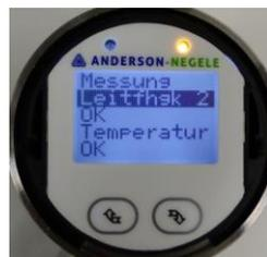
After the sensor is started, the screen saver appears in which the process values of the sensor are displayed one after the other. To reach the start page from here, press one of the two buttons briefly. Further information on operating the display can be found in the quick start manual and in the operating manual for the modular sensors (ITM-51, ILM-4, ...).
