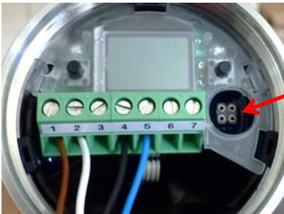
Connection plug for the MPI-200-F adapter as an intermediate plug between the ITM-51 electronics and the MPI-200 connection 3 (see the next figure).
