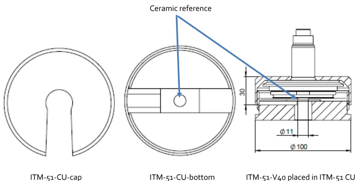
The ITM-51-CU unit is used as below:
