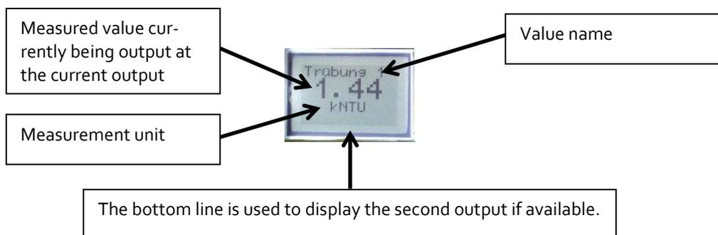
To leave the display mode and create settings on the sensor, press the right button next to the display twice to enter the menu. The sensor then displays the start page, from where the settings can be created.
