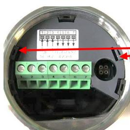
Remove the plastic cover: To do so, bend the tabs slightly inwards with a screwdriver to be able to remove the cover easily.
